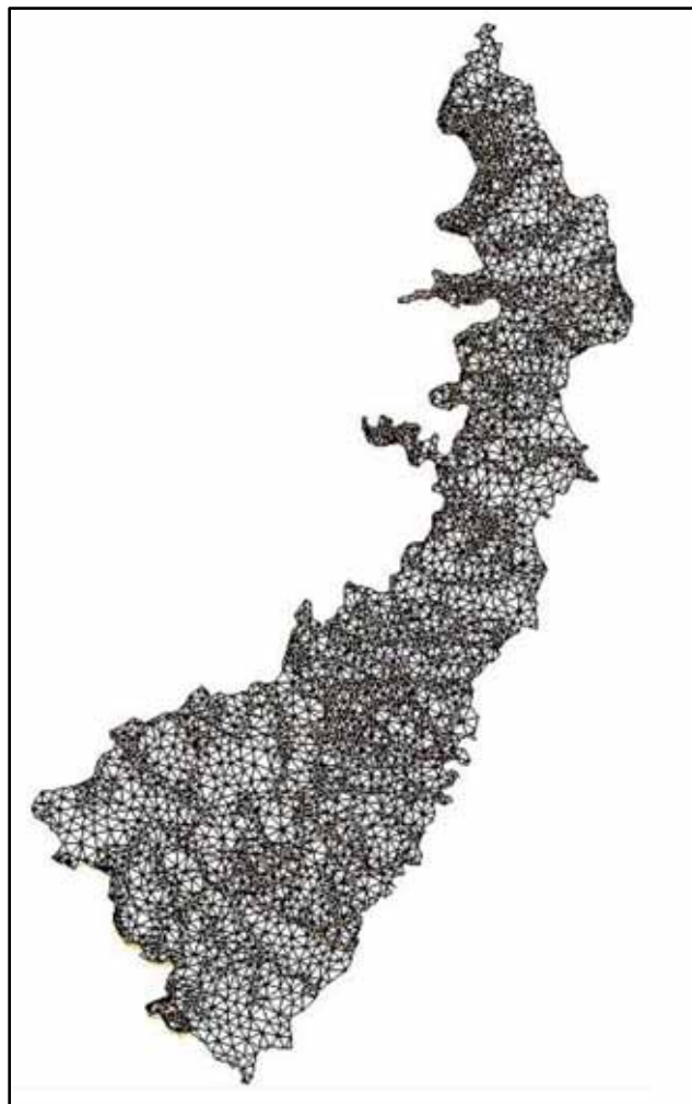
Fig. 23 Area considered for mathematical modeling, preliminary mesh in FEFLOW.
