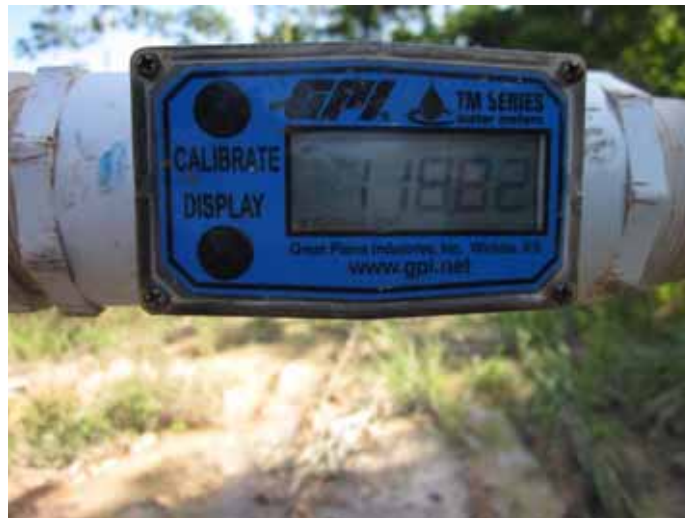
Figure 4: Flow meter utilized during hydraulic testing of HGE1
