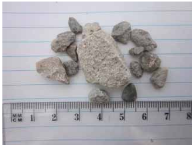
Figure 11: Conglomeratic limestone with rounded pebbles and wackestone/packstone
