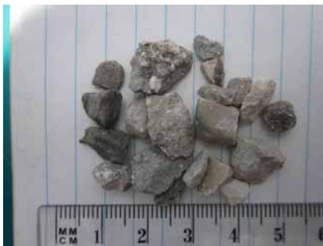
Figure 10: Conglomeratic unit with broken rounded pebbles and dark coloured lime mud
