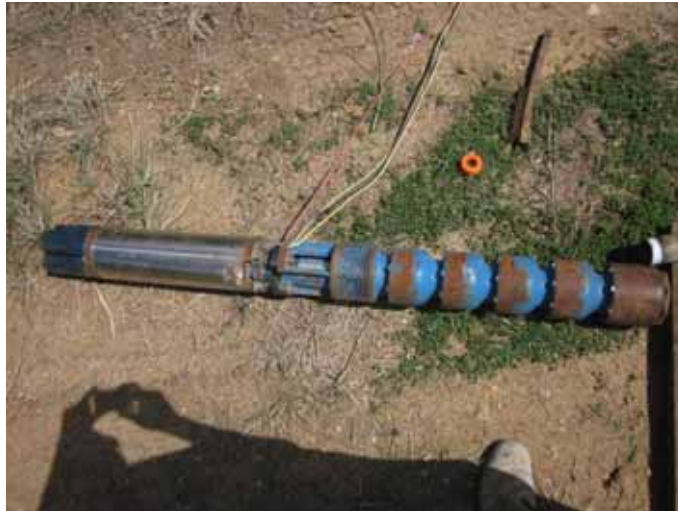
Figure 2: Submersible pump utilized for hydraulic testing of HGE-1
